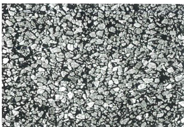
FIG. X1.34 Polished Aggregate
