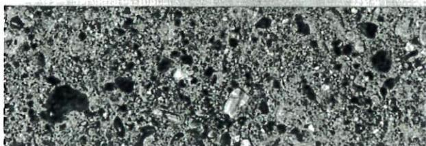
FIG. X2.31 Polished Aggregate
